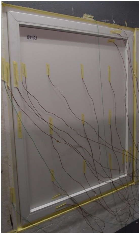
Photo of the cut test specimen frame profiles
